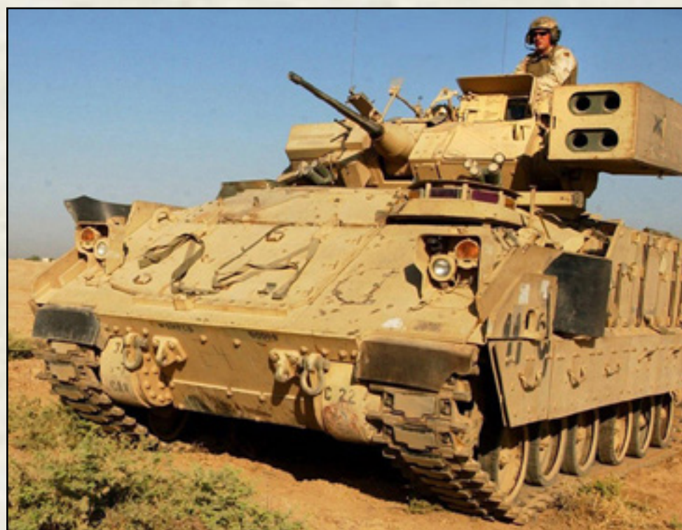
M6 LINEBACKER: An air defense variant, these vehicles are modified M2A2 ODSs with the TOW missile system replaced with a four-tube Stinger missile system.
