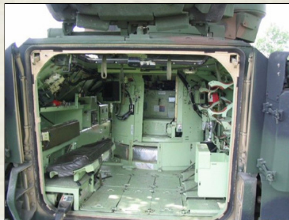
CLIMB ON BOARD: The interior of a Bradley Fighting Vehicle. It has a crew of three and can also carry six fully-equipped troops.
